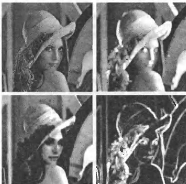
Fig.10. Original image LENA (a), image LENA - dilation (b), image LENA - erosion (c), image LENA - edge (d)
