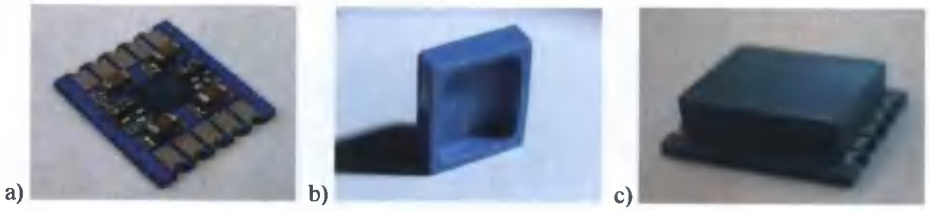
Fig. 6. Final device: a) assembled fired LTCC substrate, b) top housing part, c) housed structure
