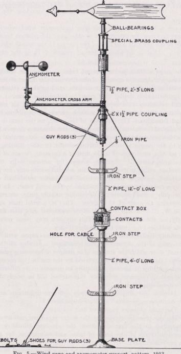
Fig. 5.—Wind vane and anemometer support, pattern, 1913.
