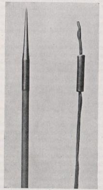
Fig. 136.—Originally duplicate hollow copper lightning rods; one never used, the other crushed by a lightning discharge.
