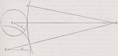
Fig. 154.—Sound ranging, or locating sound source.
