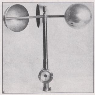
Fig. 4.—Three-cup anemometer.
