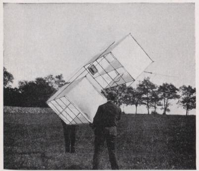
Fig. 13.—Launching meteorological kite.
