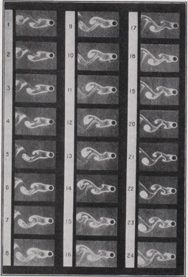
Fig. 155.—Eddies behind cylinder. (N. P. L.)
