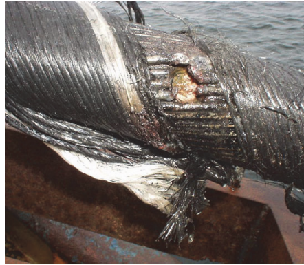
Fig. 5. Repair of the damaged return cable: a) the moment of taking out the cable from the water b) electrically damaged strands of a return cable [own source]
