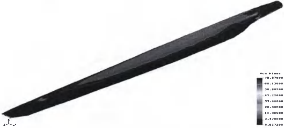
Fig. 8. Course of strength in blade epoxy- fibreglass part
