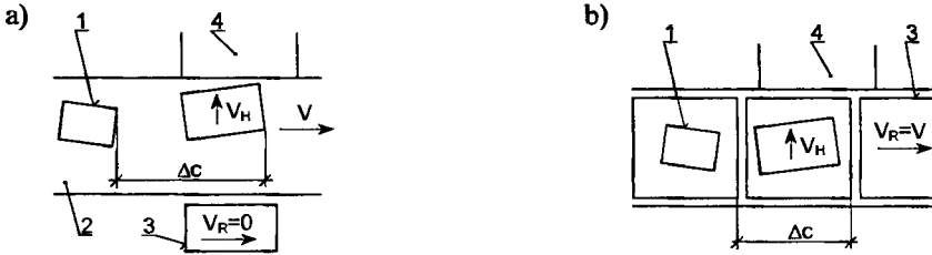
Fig. 1. Physical models of sorting machine of: a) stationary, b) streaming; 1 – load, 2 – conveyor, 3 – divider, 4 – skid, V – linear speed, V_H – speed of divider working element, \Delta c – minimal permissible distance between loads
